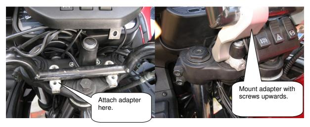
Hang out the clutch and throttle cable and put it aside so that both can be repositioned later. Fit the brake hose extension – as shown in the picture. Now the handlebar can be dismantled in order to fit both enclosed handlebar adapters.
